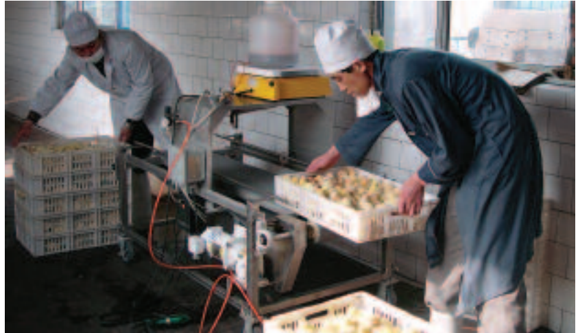
Zhucheng hatchery workers use a specially designed spray cabinet to administer coccidiosis vaccine to day-old chicks.
